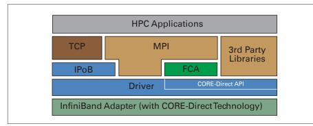
Figure 2. Software architecture with FCA and CORE-Direct
